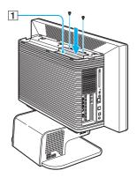
**12** Gently slide the top panel onto the computer until it snaps into place.
